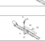
Attach 4 (steady support) to the end of main arm with 21 (plug).
